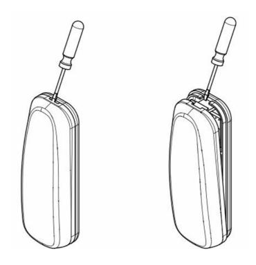
Insert 2 CR2032 batteries into the battery holder. Pay attention to the polarity.
