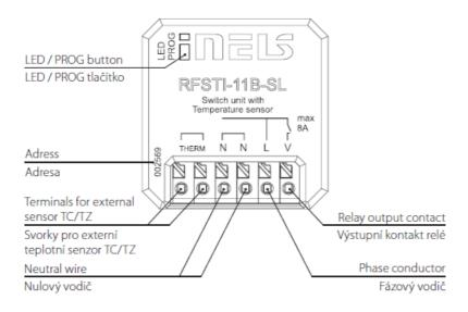
Pressing the button activates the output for 10 seconds. At this point, it is possible to check the wiring of the electrical circuit, without the need for assignment to the system.
