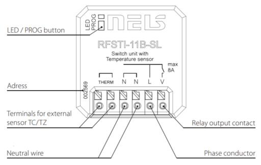
Pressing the button activates the output for 10 seconds. At this point, it is possible to check the wiring of the electrical circuit, without the need for assignment to the system.
