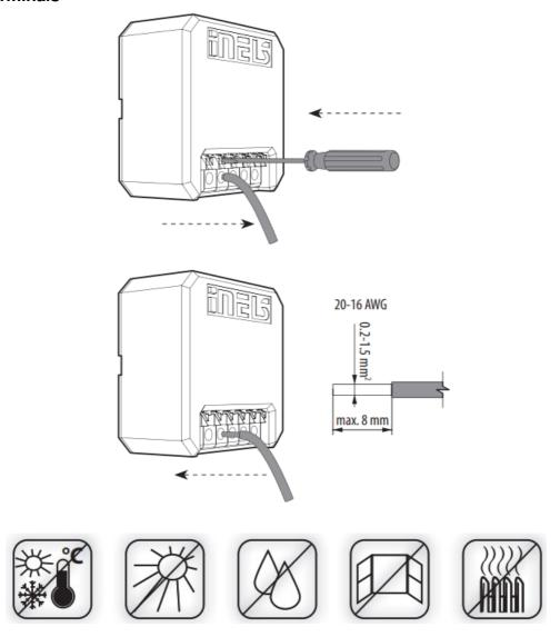
Avoid rapid temperature changes, direct sunlight and excessive moisture. The temperature units should not be located near windows or heating equipment, etc., which could affect the internal temperature sensor.
