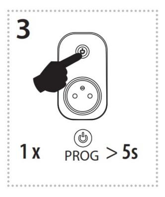
Press of programming button longer then 5 seconds, will activate actuator into timing mode. LED fl ashs 2x in each 1s interval. Upon releasing the button, the delayed return time starts counting.
