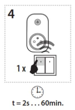
After the desired time has elapsed (range of 2s ... 60min), the timing mode ends by pressing the button on the RF transmitter, to which the delayed on function is assigned. This stores the set time interval into the actuator memory.
