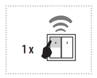
The output contact will be opened by pressing the button and closed after the set time interval has elapsed. **Programming** setting time delay 2s ... 60min.
