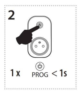
Pressing the programming button on the RFSC-61N receiver for less than 1 second will fi nish the programming mode, this will reverse the memory function. The LED lights up according to the current pre-set memory function. The set memory function is saved. Every other change is made in the same way.
