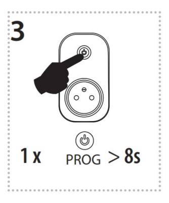
Pressing the PROG button for longer than 8 seconds brings the socket into the timing mode. The LED will give a single fl ash 3x and a double fl ash 3x, then goes out.
