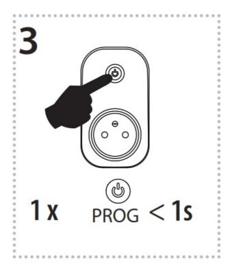
Press of programming button on receiver RFSC-61N shorter then 1 second will fi nish programming mode. The LED lights up according to the preset memory function.
