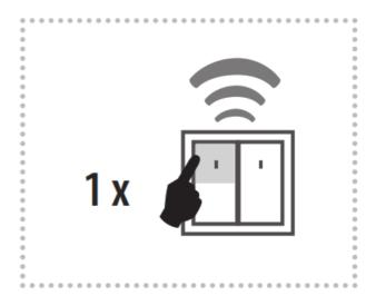
The output contact will be closed by pressing the button.
