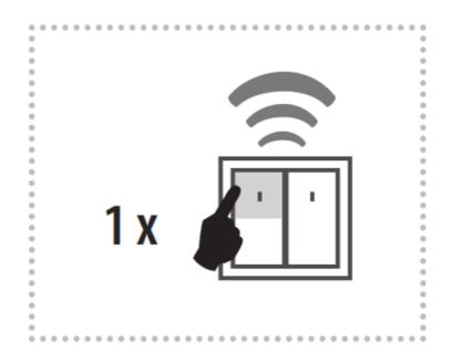
The output contact will be closed by pressing the button and opened by releasing the button. For the correct execution of individual commands (press = closing / releasing the button = opening), the time delay between these commands must be a min of.
