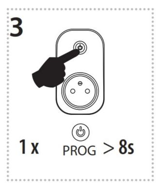
Pressing the PROG button for longer than 8 seconds brings the socket into the timing mode. The LED will give a single fl ash 3x and a double fl ash 3x, then goes out.
