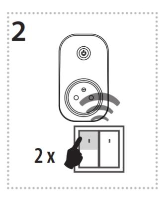
Two presses of your selected button on the RF transmitter assigns the function switch on (must be a lapse of 1s between individual presses).
