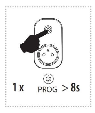
By pressing the programming button on the actuator for 8 seconds, deletion occurs of the actuator's entire memory. LED fl ashs 4x in each 1s interval.
