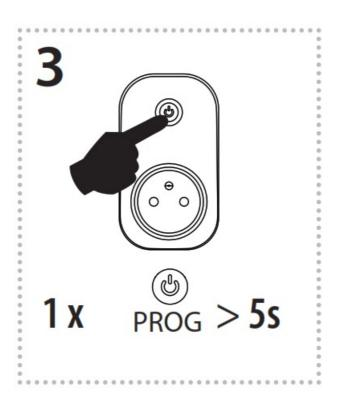
Press of programming button longer then 5 seconds, will activate actuator into timing mode. LED fl ashs 2x in each 1s interval. Upon releasing the button, the delayed return time starts counting.
