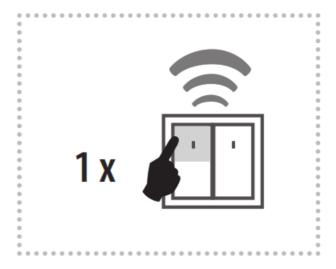
The output contact will be switched to the opposite position by each press of the button. If the contact was closed, it will be opened and vice versa.
