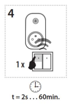
By the number of presses of the selected RF transmitter button, set the required delay (1 press - 1h, ... 10 presses - 10h). Each press on the RF transmitter is indicated by a fl ash of the LED on the socket RFSC-61N.
