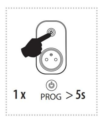
By pressing the programming button on the actuator for 5 seconds, deletion of one transmitter activates. LED fl ashs 4x in each 1s interval.
