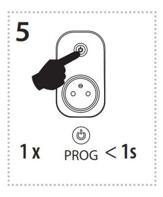
Press of programming button on receiver RFSC-61N shorter then 1 second will fi nish programming mode. The LED lights up according to the preset memory function.
