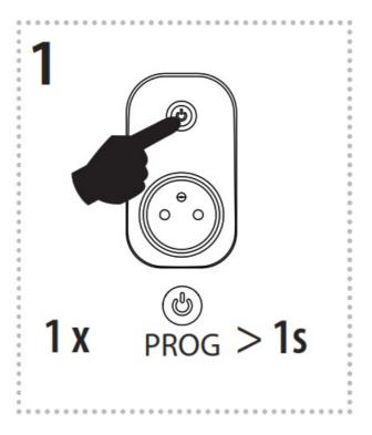
Press of programming button on receiver RFSC-61N for 1 second will activate receiver RFSC-61N into programming mode. LED is fl ashing in 1s interval.
