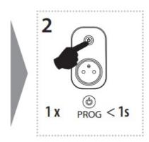
Pressing the programming button on the RFSC-61N receiver for less than 1 second will fi nish the programming mode, this will reverse the memory function. The LED lights up according to the current pre-set memory function. The set memory function is saved. Every other change is made in the same way.
