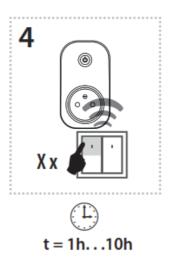
By the number of presses of the selected RF transmitter button, set the required delay (1 press - 1h, ... 10 presses - 10h). Each press on the RF transmitter is indicated by a fl ash of the LED on the socket RFSC-61N.
