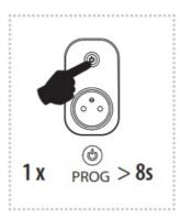
By pressing the programming button on the actuator for 8 seconds, deletion occurs of the actuator's entire memory. LED fl ashs 4x in each 1s interval. The actuator goes into the programming mode, the LED flashes in 0.5s intervals (max. 4 min.). You can return to the operating mode by pressing the Prog button for less than 1s. The LED lights up according to the pre-set memory function and the component returns to the operating mode. Deletion does not affect the pre-set memory function.
