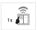
The output contact will be closed by pressing the button and opened after the set time interval has elapsed. **Programming** setting time delay 2s ... 60min.
