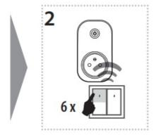
Assignment of the delayed on function is performed by six presses of the selected button on the RF transmitter (must be a lapse of 1s between individual presses).
