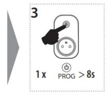
Pressing the PROG button for longer than 8 seconds brings the socket into the timing mode. The LED will give a single fl ash 3x and a double fl ash 3x, then goes out.
