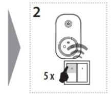
Assignment of the delayed off function is performed by fi ve presses of the selected button on the RF transmitter (must be a lapse of 1s between individual presses).
