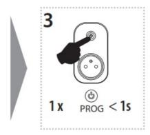
Press of programming button on receiver RFSC-61N shorter then 1 second will fi nish programming mode. The LED lights up according to the preset memory function.
