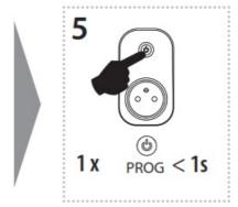
Press of programming button on receiver RFSC-61N shorter then 1 second will fi nish programming mode. The LED lights up according to the preset memory function.
