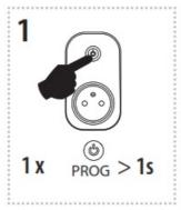
Press of programming button on receiver RFSC-61N for 1 second will activate receiver RFSC-61N into programming mode. Red LED is flashing in 1s interval.
