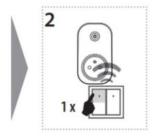
Select and press one button on wireless switch, to this button will be assigned function Button.
