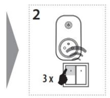
Three presses of your selected button on the RF transmitter assigns the function switch off (must be a lapse of 1s between individual presses).
