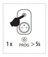
By pressing the programming button on the actuator for 5 seconds, deletion of one transmitter activates. LED fl ashs 4x in each 1s interval. Pressing the required button on the transmitter deletes it from the actuator's memory. To confi rm deletion, the LED will confi rm with a fl ash long and the component returns to the operating mode. The memory status is not indicated. Deletion does not aff ect the pre-set memory function.
