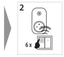
Assignment of the delayed on function is performed by six presses of the selected button on the RF transmitter (must be a lapse of 1s between individual presses).
