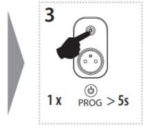
Press of programming button longer then 5 seconds, will activate actuator into timing mode. LED fl ashs 2x in each 1s interval. Upon releasing the button, the delayed return time starts counting.
