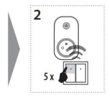
Assignment of the delayed off function is performed by fi ve presses of the selected button on the RF transmitter (must be a lapse of 1s between individual presses).
