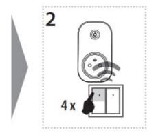
Four presses of your selected button on the RF transmitter assigns the function impulse relay (must be a lapse of 1s between individual presses).
