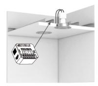
mounting into the light cover ceiling mounted
