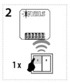
3. Press of the programming button on receiver RFSAI-62B shorter than 1 second will finish programming mode. The LED lights up according to the pre-set memory function.
