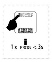
Channel selection (RFSAI-62B-SL) is done by pressing the PROG buttons for 1-3s. RFSAI-61B-SL: press for more than 1 second. After the button release, LED is fl ashing indicating the output channel: red (1) or green (2). All other signals are indicated by the corresponding color of the LED for each channel.
