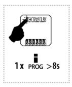
Pressing of the programming button on receiver RFSAI-62B for 3-5 seconds (RFSAI-61B-SL: press for 1 second) will activate receiver RFSAI-62B into programming mode. LED is fl ashing in 1s intervals.
