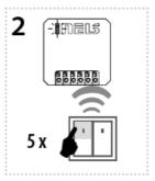
1. Pressing of the programming button on receiver RFSAI-62B for 3-5 s (RF-SAI-61B-SL: press for more than 1 s) will activate receiver RFSAI-62B into programming mode. LED is fl ashing in 1s intervals.
