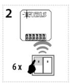
3. Pressing of the programming button for longer than 5 seconds will activate the actuator into timing mode. LED flashs 2x in each 1s interval. Upon releasing the button, the delayed return time starts counting.
