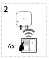
• Press of the programming button longer than 5 seconds, will activate the actuator into timing mode. LED flashes 2x in each 1s interval. Upon releasing the button, the delayed return time starts counting.
