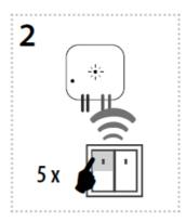
• Press of the programming button longer than 5 seconds, will activate the actuator into timing mode. LED
