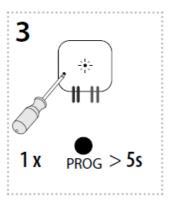
• After the desired time has elapsed (range of 2s...60min), the timing mode ends by pressing the button on the RF transmitter, to which the delayed return function is assigned. This stores the set time interval into the actuator memory.
