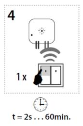
Press of the programming button on receiver RFSAI-61B shorter then 1 second will finish programming mode.
