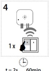
• Press of the programming button on receiver RFSAI-61B shorter than 1 second will finish programming mode. The LED lights up according to the pre-set memory function
