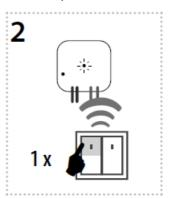
Press of the programming button on receiver RFSAI-61B shorter than 1 second will fi nish programming mode.
