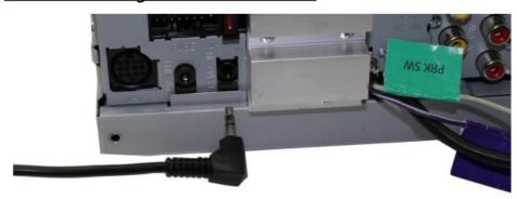
4. Connect the 14 way molex connector to the interface.
