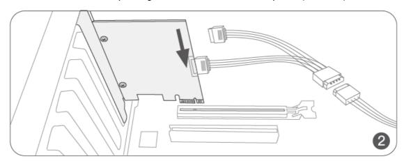
• Use the screws included or the screws of the computer case to fix the PCI-E card.
