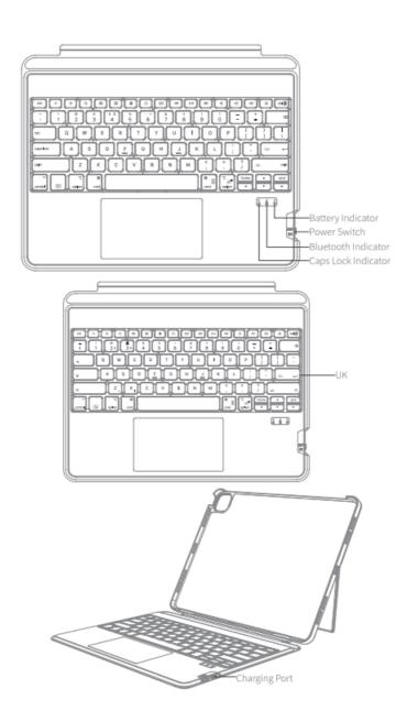
Step 1: Put the iPad case on and slide the keyboard switch to the On position. Hold down simultaneously and then the keyboard will enter pairing mode with a blinking blue indicator light. Step 2: On your iPad, go to Settings > Bluetooth, turn on Bluetooth and then "Inateck KB04118" will showupin "Other Devices". Step 3: Tap "Inateck KB04118" to pair it with your iPad. The Bluetooth indicator will go off in seconds, which means that Bluetooth pairing is completed.
