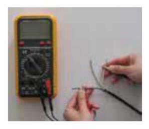
Resistance must be measured between the white and black conductors using an ohmmeter or multimeter. Compare the resistance measurement with the one printed on the product's label. If the multimeter is manual, adjust it to the 200-Ohm setting.
