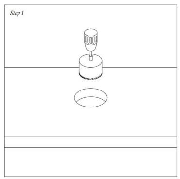
Drill out a 2 1/2" diameter hole to fit the threaded base column.
