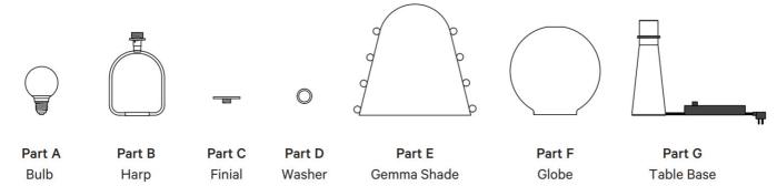
Step 1: Slide the glass globe (F) over the table base (G). Align the sidehole on the glass base with the cord.
