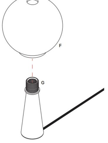
Step 2: Thread washer (D) onto table base, tightening the globe (F) into place.
