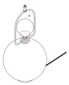
• Step 5: Carefully place Fazzo shade (E) onto the harp (B), feeding the threaded part through the hole in the shade.
