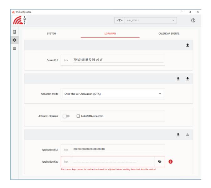
Now a first test if the network can be reached by iO881A can be started. Therefore start the activation of the LoRaWAN stack by moving the slide switch to the right side. iO881A than starts the joining procedure. You can check either on the network server side if the corresponding "Join Requests" are received by the network server or observe the LED signalling of iO881A.
