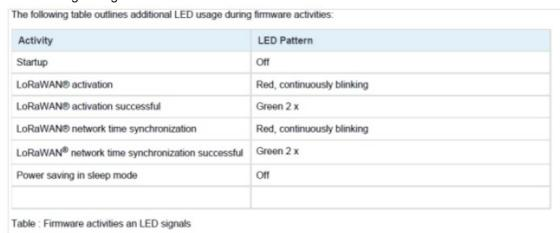
Now you can close the "WS Configurator", and unplug the USB cable from your laptop. Connect the USB cable of the iOKE868 to your preferred power supply (USB battery pack or USB power plug). Observe the LED signalling of the iO881A during start up, refer to the table above.
