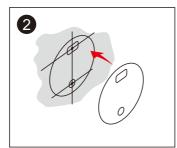
2.Cover mounting bracket paper on marked circle base, mark 2 points according to paper holes to drill wall holes.
