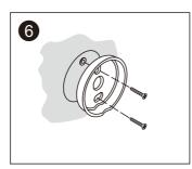
6. Use screwdriver tighten the mounting bracket on wall stable.
