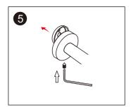
5.Use allen wrench loosen the setting screw and remove the mounting bracket from accessory.
