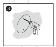
3. Use 1/4 inch driller to drill holes on wall which you marked, the depth same as white anchor.
