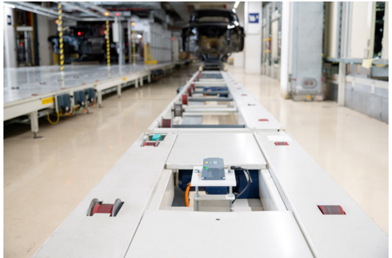
For reliable vehicle identification, the RFID system SIMATIC RF300 is used.
