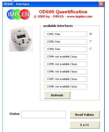
Step 4: Click the "Read Values" button. The message "Press 'OK' and then press 'print' on the device within 20 seconds" will appear. Press OK and then press the recall/print button on your OD600 DiluPhotometer™. The memory (MEM) number on the display of your OD600 DiluPhotometer™ is flashing during data transfer.
