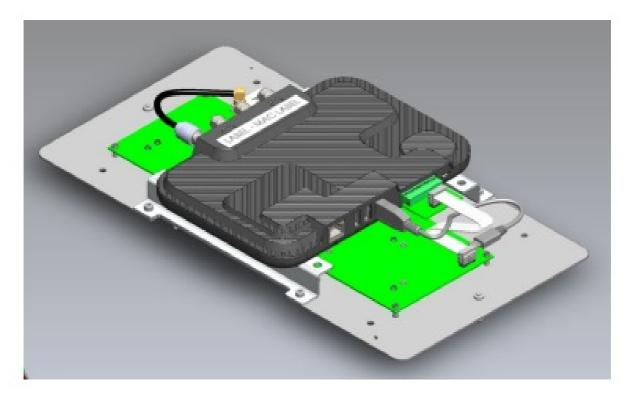
• The reader features multiple interfaces. Ethernet network interface, USB ports and GPIO block are located on the end of the reader. The Ethernet network jack is the only interface that the customer is required to access.
