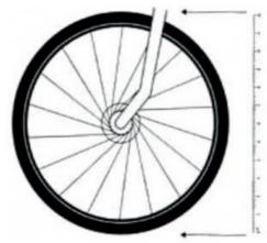
Following the example above, enter the number '2154' on the speedometer. Press the **RIGHT** button to increase the value of the digits and the **LEFT** button when you want to confirm the figure and keep moving forward. (Range of circumference O mm - 9999 mm). Press the LEFT button to enter the **KM/M** mode.
