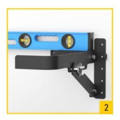
2. Set the base at the desired height, and use a torpedo level to ensure the base is horizontal so the stands will have a level surface to rest on. Use the base as a template to mark the location of the holes in the surface.
