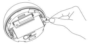
3. Hold down the Set button for 5 s until the LED flashes green to enter the pairing mode.
