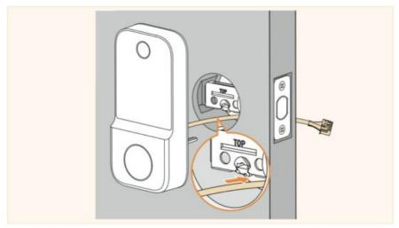
2. Position the tailpiece horizontally and insert it into the slot of the latch.
