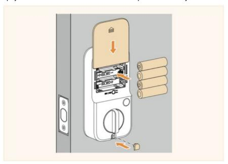
• After installation, rotate the thumbturn to test if the deadbolt can move freely. The rotation direction depends on the door's opening and here is presented for lefthanded doors.
