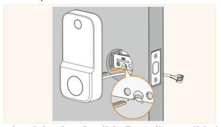
3. Attach the mounting plate to the inner door surface with the silicone pad in contact with the door. Guide the cable and tailpiece through their respective holes on the mounting plate.
