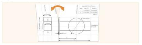
2. Attach the drilling template to the door. Make sure the center lines are aligned.
