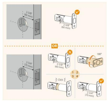
2. Inset the latch into the designated hole with the TOP mark on the latch facing up.
