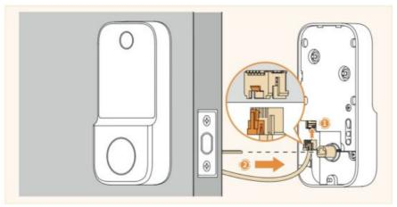
2. Secure the indoor panel with No. L screws.
