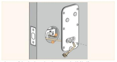
4. Keep the mounting plate parallel to the door edge, then secure it with No. K screws.
