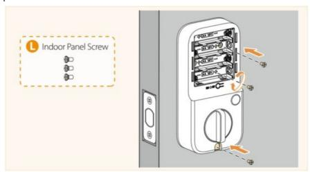
3. Install batteries and pay attention to the terminal orientation. Replace the battery cover and the plug.
