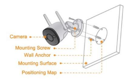
Step1 Drill screw holes on the mounting surface as the positioning map shows, and then put in the wall anchors. Step2 Attach the pedestal to the mounting surface with the mounting screws. Step3 Power up the camera, and then adjust the lens to the ideal angle.
