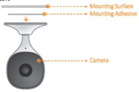
Sten 1 Peel off the mounting adhesive and stick it to the bottom of the camera.
