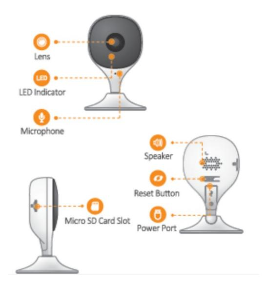
Press and hold the reset button for 10 s to reset the camera. See the table below for definitions of the camera's LEO behaviors.
