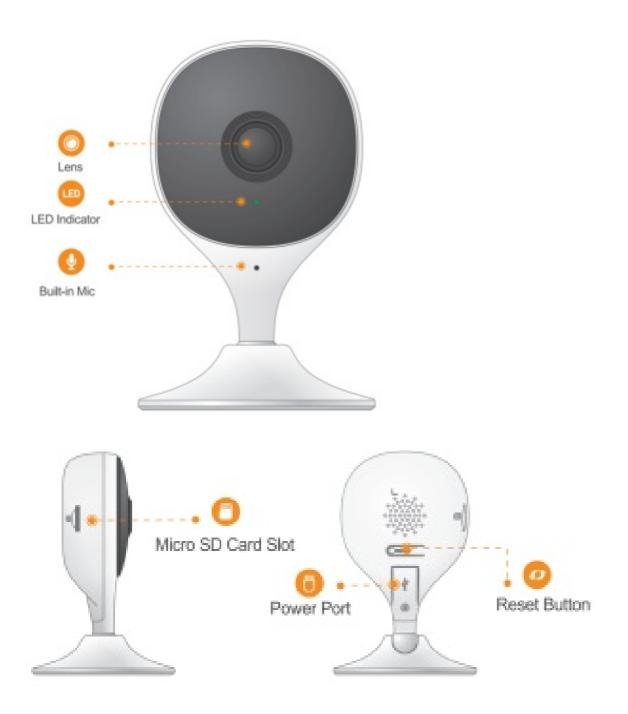
**Note:** Press and hold the reset button for 10 s to reset the camera. The pattern of the LED indicator is included in the following table.
