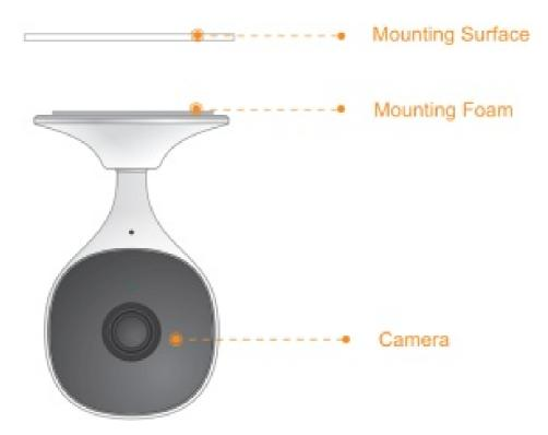
Step 1 Stick the mounting foam on the camera pedestal.
