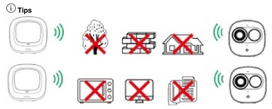
To ensure the best possible wireless performance, please make sure there are no obstacles and electromagnetic interference between the camera and hub.
