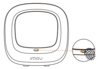
2. Press the SYNC button, and then the indicator on the camera flashes with green light.
