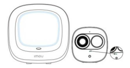
**Note:** You can pair six cameras at most with one Hub, and pair one camera at a time. Keep the distance of the Hub and the camera within 30 cm (12 inches)during pairing.
