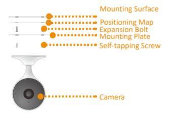
Step 1 Drill screw holes on the mounting surface as the positioning map shows, and then put in the expansion
