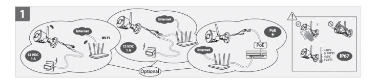
• Connect the camera to power. You can choose a wireless or wired network connection. Since the camera is PoE-featured, you can also connect it to a POE device such as a POE switch with an Ethernet cable to transmit both power and data (see part 1).
