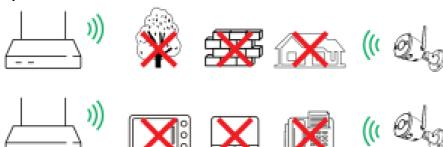
To ensure the best possible wireless performance, please make sure there are no obstacles and electromagnetic interference between the camera and router.
