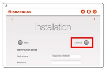
After entering the device name and password, press "Continue" (Fig. 3) to access the "Connectivity Settings" screen (Fig. 4). From the screen below, enter the following data:
