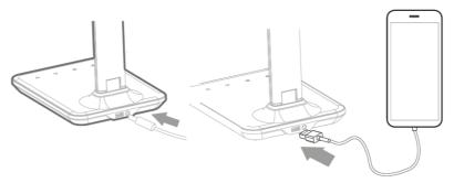
USB connector: DC5V / 1A – this connector is intended only for mobile devices or accessories with a consumption lower than 5V / 1A.
