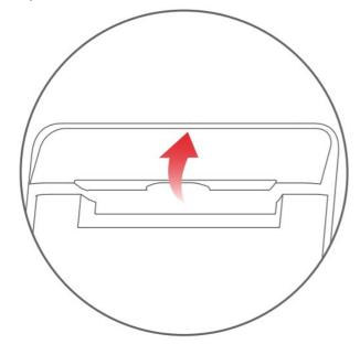
2. Turn the rotary knob of cutter up until the paper jam is removed
