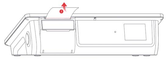
3. After printing, tear the paper upwards.
