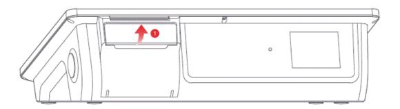
1. Unscrew the printer cover and the paper compartment door pops open;
