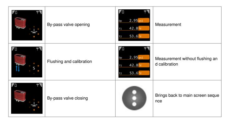
\*) Keeping pressed from the start keeps the calibration sequence in flushing phase. Flushing phase is ended by releasing
