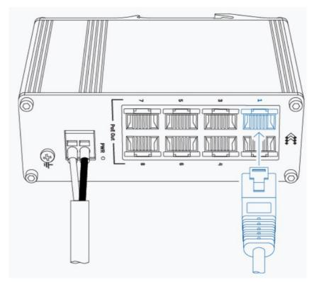
3. Connect the end devices to the Ethernet ports numbered 1 to 8.
