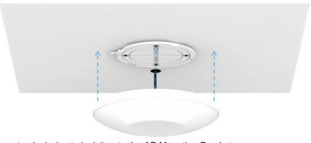
4. Turn the TAP200 counterclockwise to lock it onto the AP Mounting Bracket.
