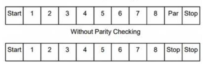
Even parity is required, other modes (odd parity, no parity) may also be used. In order to ensure a maximum compatibility with other products, it is recommended to support also No parity mode. The default parity mode must be even parity. Remark: the use of no parity requires 2 stop bits.
