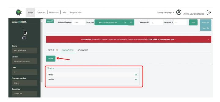
Press Check to verify the correct communication between the LoRaWAN® interface and the slave(s).
