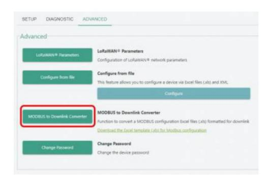
**MODBUS to Downlink converter:** convert the .XLS configuration file in one or more downlink payload to be sent to the device instead using USB port-.
