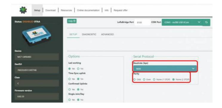
**Baud rate [bps]:** set the baud rate for the serial line (defalt = off).
