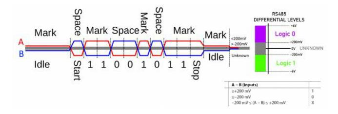
The objective of biasing is to make sure that the RS485 line remains in a known, non-fluctuating state when no devices are transmitting. Polarization of the pair must be implemented at one location for the whole serial bus. Biasing the entire network requires a single pair of polarization resistors: a pullup resistor to +5V attached to the "+" signal line, and a pull-down resistor to ground attached to the "-" signal line.
