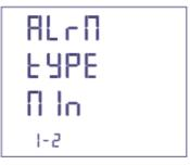
Quantity that can be coupled: phase voltage (L1-N, L2-N, L3-N) interlinked voltage (L1-L2, L2-L3, L3-L1) phase current (11, 12, 13) frequency
