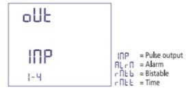
The output relay (terminals 15-29) can be used as energy pulses (see point 1.7a) repeater or as alarm relay (see point 1.7b) or as remote-controlled state of relay switching (see point 1.7c- point 1.7c).
