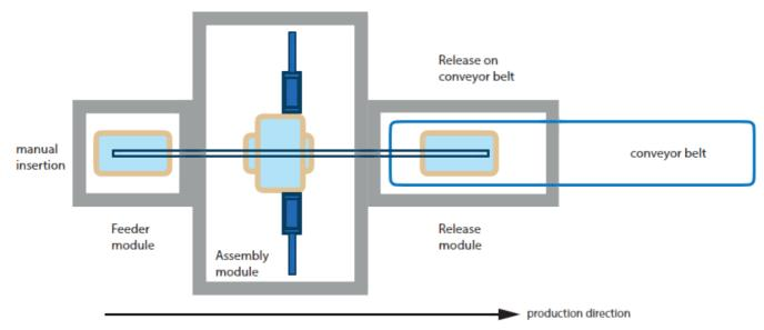
fastFrame 600 SA is a fully automated multi-format system for industrial high-speed stretching of canvases. It mounts up to 163 canvases per hour, depending on the size and operator skills. This is way faster than manual production.
