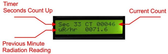
tion level for one second before beginning another CPM counting cycle. If you change to the 1 minute time from 1 second the second line will display the radiation level last calculated from the previous mode. If the Geiger counter is turned on in the 1-minute mode the second line will display the word "Initializing" for the first 60 seconds.
