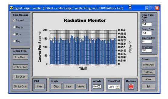
onds, Minutes, Hours, or Days). The recorded data can be saved and exported as a CSV delimited file for use in various other applications including Word & Excel. Data can be displayed as 1 of 4 types of graphs. One can also set alarm levels for CPS/Radiation Levels. If the values cross the specified levels, the software issues a visual and an audible alert.
