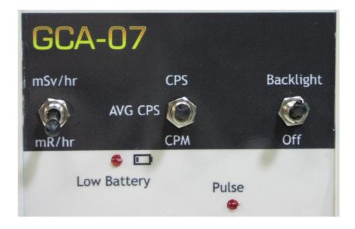
The middle switch labeled CPS, AVG CPS, and CPM selects one of the three Survey Meter Modes:
