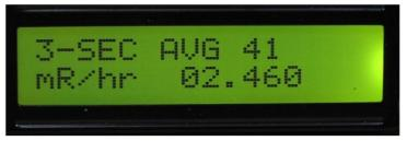
• CPM (Counts Per Minute) is a one-minute counting mode for measuring low levels of radioactivity and background radiation: Displays accumulated count and equivalent background radiation in either uR/hr or uSv/hr. If the radiation level is significant radiation level is displayed in either mR/hr or mSv/hr.
