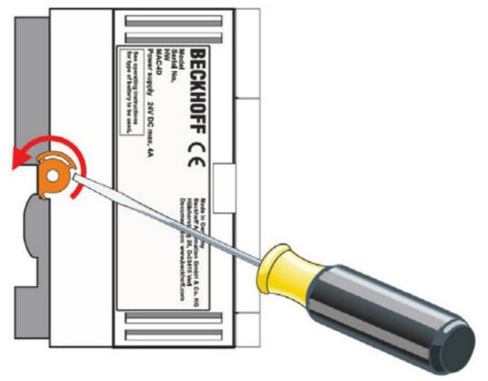
3. Double-check the correct installation and latching of the contact closure module on the mounting rail.
