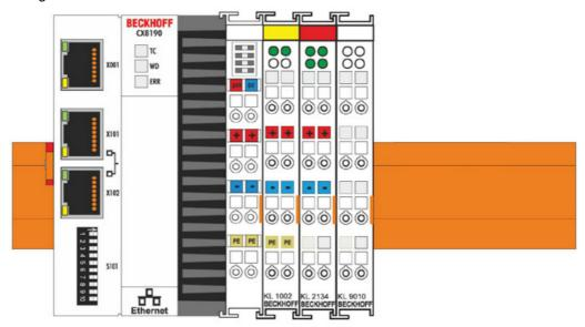
2. Subsequently, lock the catch on the left side of the contact closure module.
