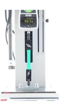
This unit graphs the process and enables you to visually check the force transition until the sample is broken. Al so, it helps you to easily find the force/displacement value and peak value when the sample is broken, and leav e a comment.
