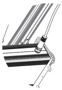
Once all the LED bars are fastened into place and A/C cables are attached to the mast, turn the fixture over (this may require more than one person). Ensure the flat surface is clear of anything that could damage the delicate diodes.
