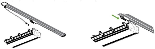
2. Once the plastic clips are all snapped in place, attach the A/C cables coming from the mast to each LED bar by aligning the connector pins and pressing the ends together. Lock by twisting in opposite directions.
