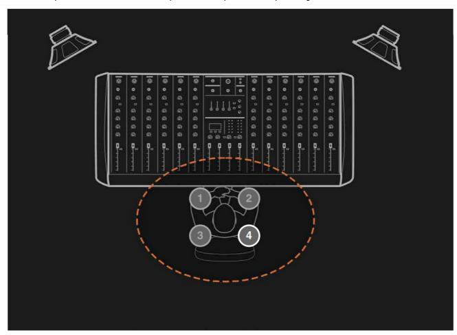
**IMPORTANT**: during the measurement process make sure that the environment is as silent as possible, do not touch the speaker or the microphone, and make sure that the overall room setup is as similar as possible to the one that will be used during normal iLoud Precision usage.
