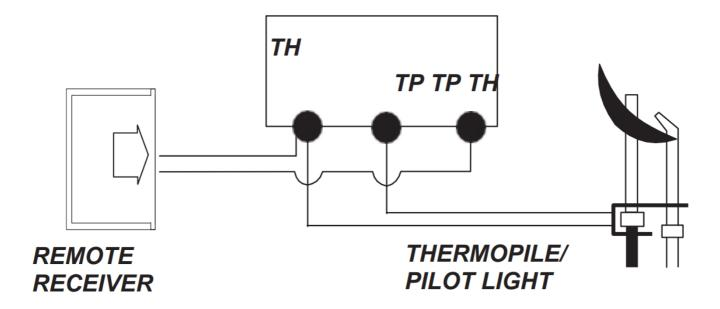
Operation of the remote receiver is similar to that of a thermostat in that both turn the gas valve ON and OFF based on input signals. A thermostat's input signals are different temperatures. The remote receiver's input signals come from the transmitter.
