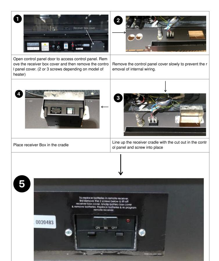
Put the control panel cover back into place
