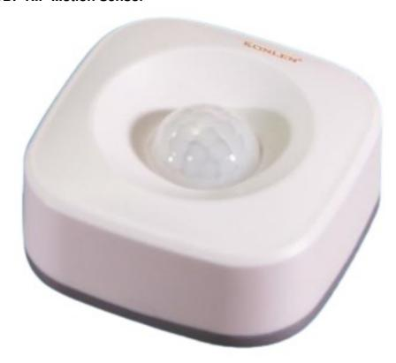
The ILLUMRA® PIR Motion Sensor detects motion and links directly to controllers such as the ILLUMRA® LED Dimmer, ILLUMRA® ON/OFF Controllers, etc. The ILLUMRA® PIR Motion Sensor offers hands-free convenience by turning lights On when entering closets, bathrooms, and other areas and saves energy by automatically turning lights OFF after an adjustable timeout when no motion is detected. An integrated light sensor can be configured to keep lights off when natural light is available.
