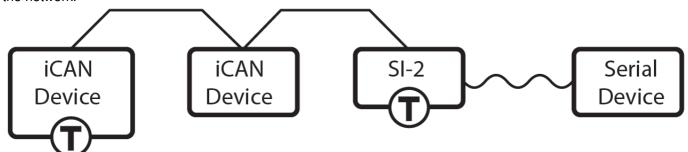
The SI-2-D unit is supplied with termination disabled as standard. If it is connected as an end device in the iCAN network, you need to move the jumper to enable termination.
