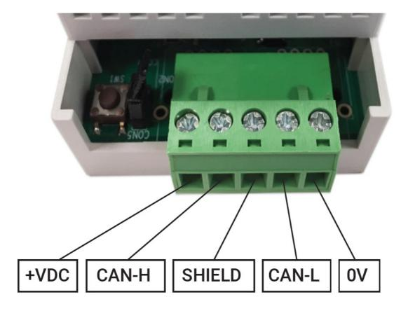
• Cable connections to the iCAN network are made to a removable 5-way connector block located at one end of the SI-2-D unit:
