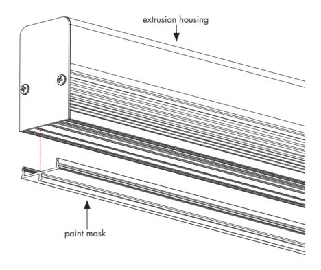
**NOTE:** Use paint mask to protect extrusion housing when doing a surface/ wall finishing. Install plexineon fixtures after removing paint mask.
