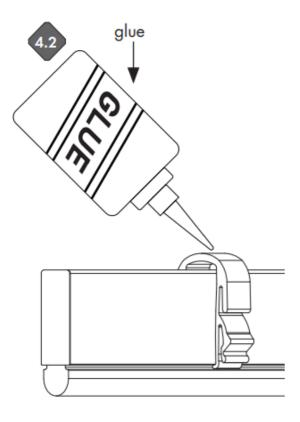
Use gule to fill in all gaps between recessed mounting clips and plexineon fixture
