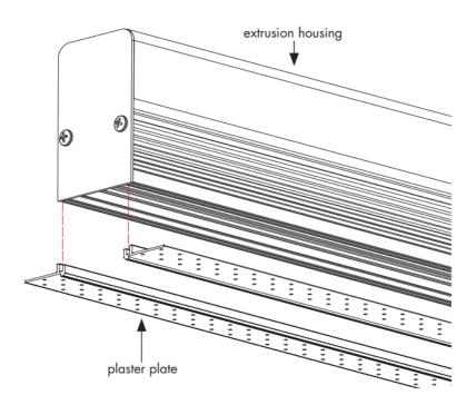
**NOTE:** Use plaster plate when doing a mud-in installation. Use paint mask to protect extrusion housing during surface/wall finishing.
