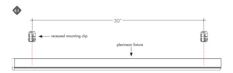
Install recessed mounting clips to fixture. Make sure they are approximately 30" apart .
