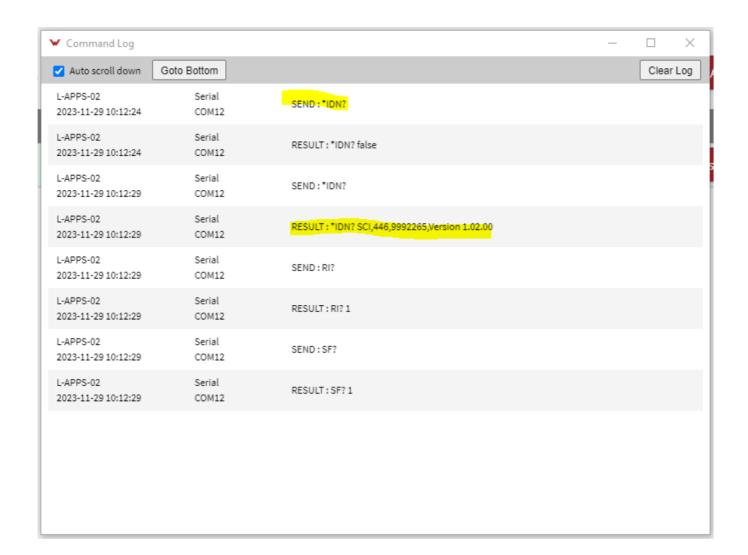
Here you can see the Withstand application querying your PC/Network for "\*IDN?" which looks for an Ikonix instrument and requests serial numbers and other identifying data. It may read false for 5-10 minutes, but this signals that the application is working. Once the instrument is found, you will be able to select the com port in the Add Instrument window.
