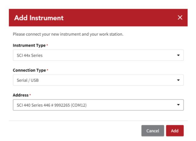
• The first instance of connecting your unit may take longer than expected (5-10min). Your PC is querying comports at different baud rates to ensure all units on PC/Network are discovered. To monitor this action a user can right click on Withstand toolbar icon and open the "Command Log" window.
